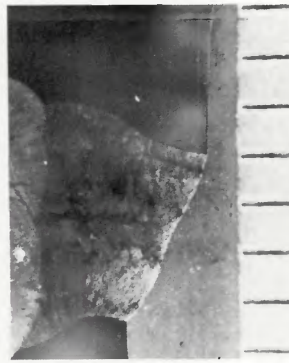
Fig. 8 - Weld UG 14(100)-13, large ID on bottom, 2G position, zero root opening, 1.59 mm (1/16 in.) mismatch. 1 mm scale (reduced 41% on reproduction)
