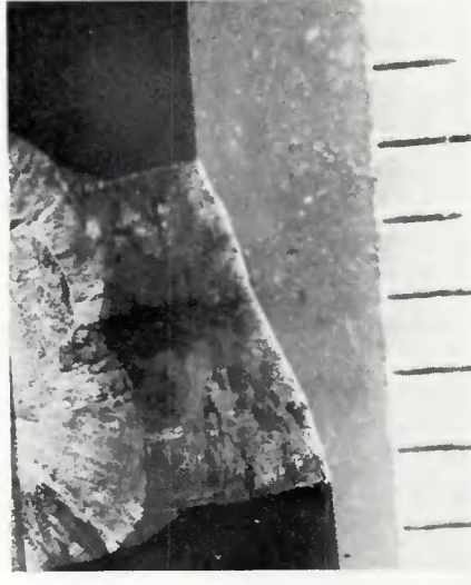
Fig. 14 - Weld UG 14(100)-11, large ID on top, 2G position, 0.79 mm (1/32 in.) root opening, 1.59 mm (1/16 in.) mismatch. 1 mm scale (reduced 41% on reproduction)
