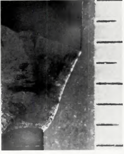
Fig. 13 - Weld UG 14(100)-9, large ID on bottom, 2G position, 0.79 mm (1/32 in.) root opening, 1.59 mm (1/16 in.) mismatch. 1 mm scale (reduced 41% on reproduction)
