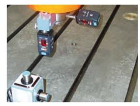
High accuracy guaranteed Machining centres geometry and accuracies are granted by the use of laser systems both in CMS and at customer premises.
