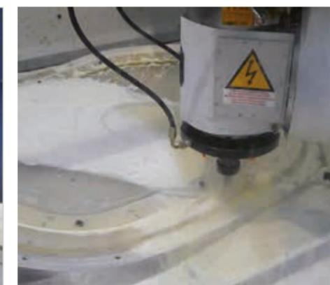
**High speed cutting CNC machine for trimming, drilling and finishing aircraft components in carbon fiber, Kevlar, composite reinforced material and Glare**
